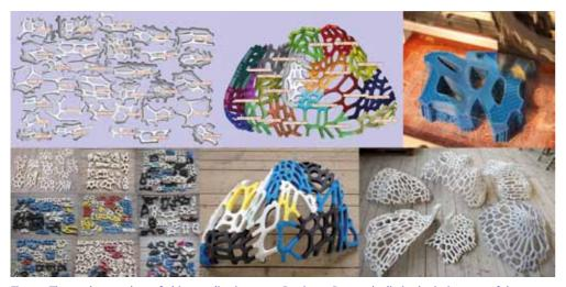
Fig. 120 The work procedure of object realisation on a 3D printer. Due to the limited printing area of the cur rent 3D printers, the object was cut into 360 pieces which were printed one by one, and put back together creating a large object, which cannot be printed at once just yet. Photo from the archive of the author
