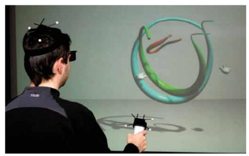
Fig. 146 Virtual environment: the user wears reflexive marks, and uses control devices and polarised glasses for interaction with VE. A projection wall with the image of three motion trails can be seen in the background
